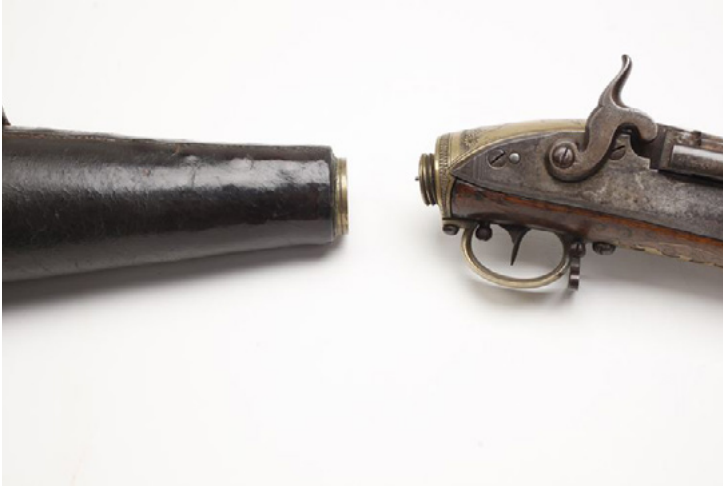
Even the 1780-era Girandoni used a detachable gas reservoir so users could change to a fresh one in the field. Photo: National Firearms Museum
